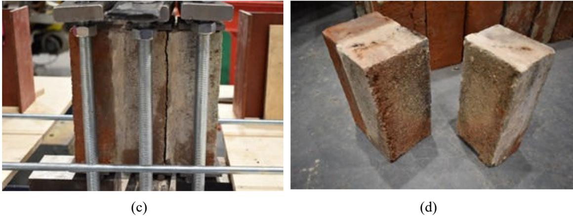
Figure 17. (a, b) Monotonic (c, d) Cyclic shear test of mortar triplets with 0.6 MPa pre-compression
