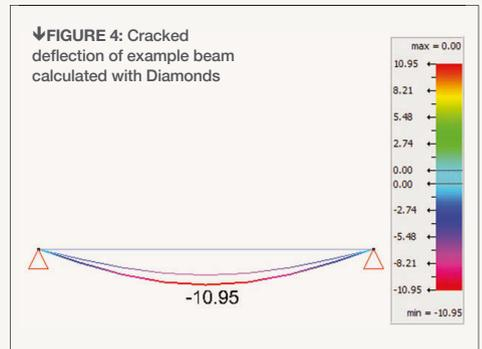
For reinforced concrete elements, the curvature value  $1/r$  depends on whether or not the cross-section is cracked. A cross-section is cracked only when the bending moment exceeds the cracking moment  $M_r$ . The cracking moment  $M_r$  is determined by
