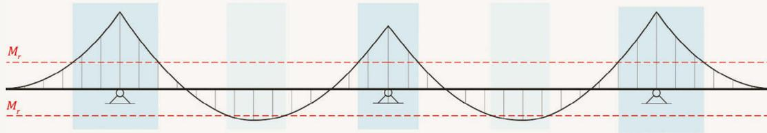
←FIGURE 2: Distribution of cracked zones in continuous beam
