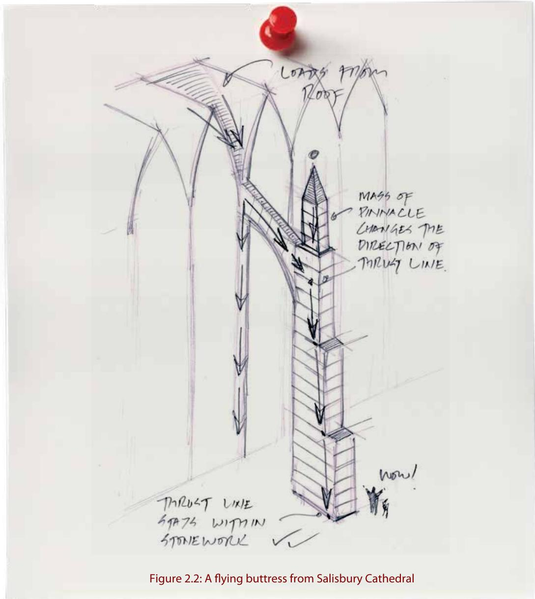
Figure 2.2: A flying buttress from Salisbury Cathedral
