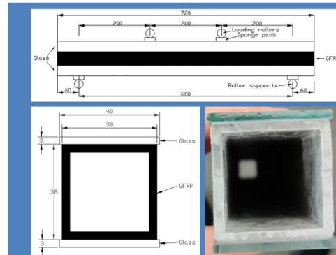
**Fig. 9:** Sandwich beam with two 3 mm thick CS glass skins on either side
