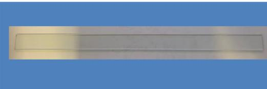
**Fig. 3:** Thin CS glass beam specimens purchased from a commercial supplier
