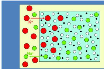
**Fig. 1:** Replacing smaller Na<sup>+</sup> with larger K<sup>+</sup>, compressive residual stresses can be introduced in glass
