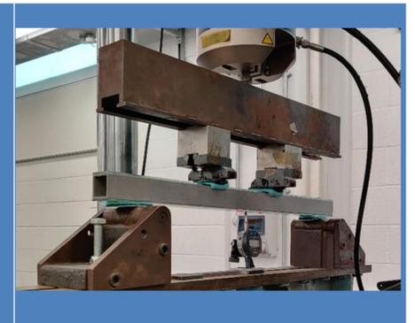
**Fig. 10:** Four-point testing of CS glass–GFRP sandwich beams
