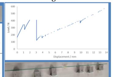
**Fig. 15:** Load-deflection relationship & failure mode
