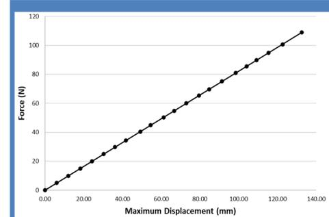
**Fig. 11:** Applied load vs midspan (i.e. maximum) deflection relationship for 3 mm thick single layer beam
