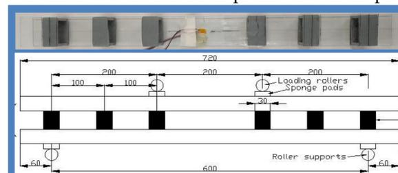
**Fig. 14:** Beam & testing arrangement of sandwich beams with intermittent GFRP rings
