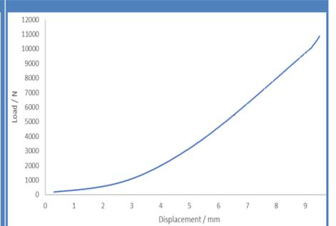
**Fig. 12:** Applied load vs midspan (i.e. maximum) deflection relationship for sandwich beam with 3 mm thick glass
