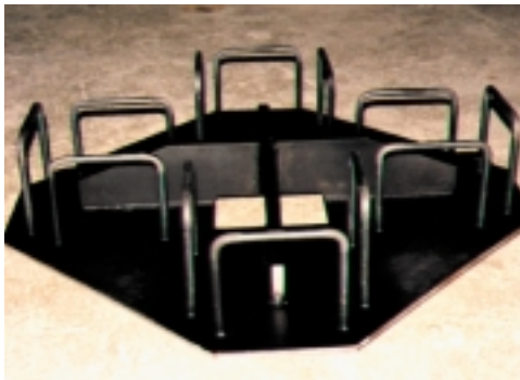
Fig 1(a) Detail of NUUL system connection
