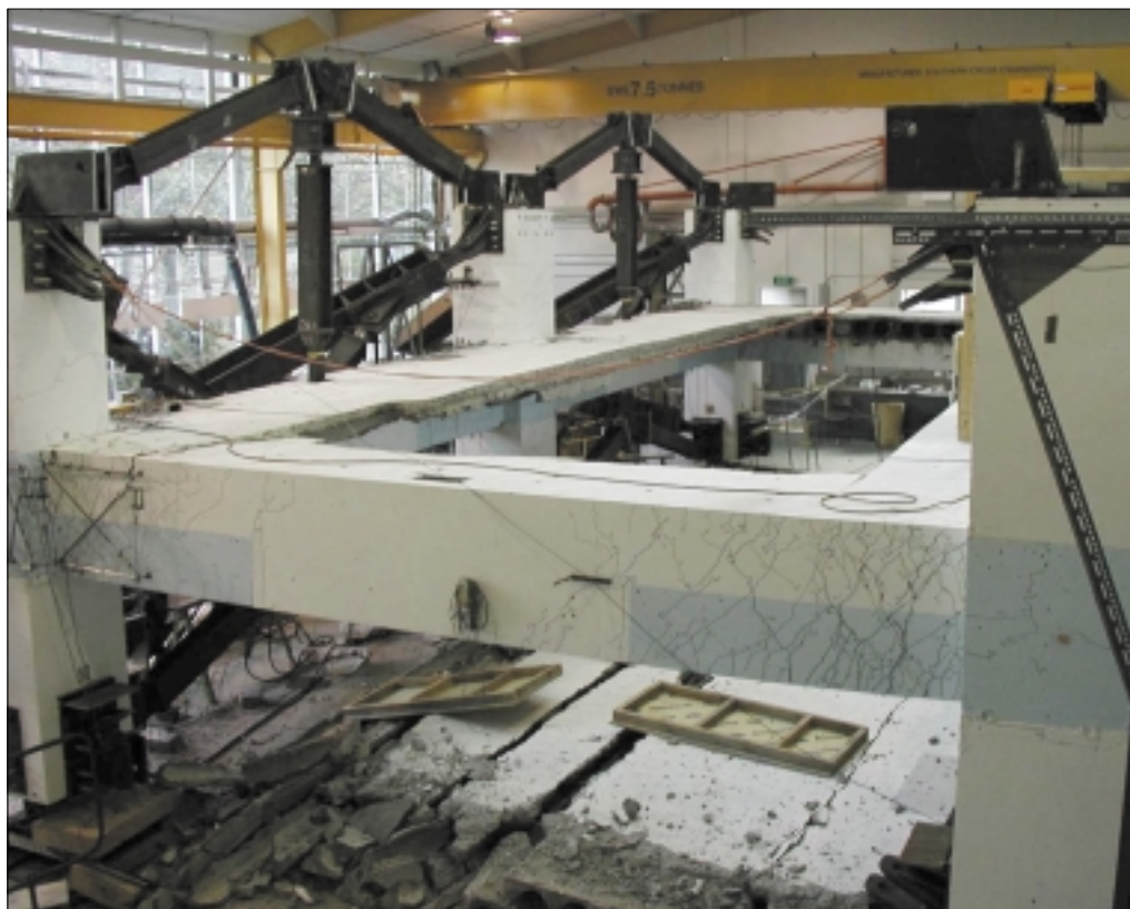
Fig 1. View of test unit from the Northeast corner after testing was completed. The steelwork on the three southern columns (part of the perimeter frame) was used to rack the unit in the East-West direction.
