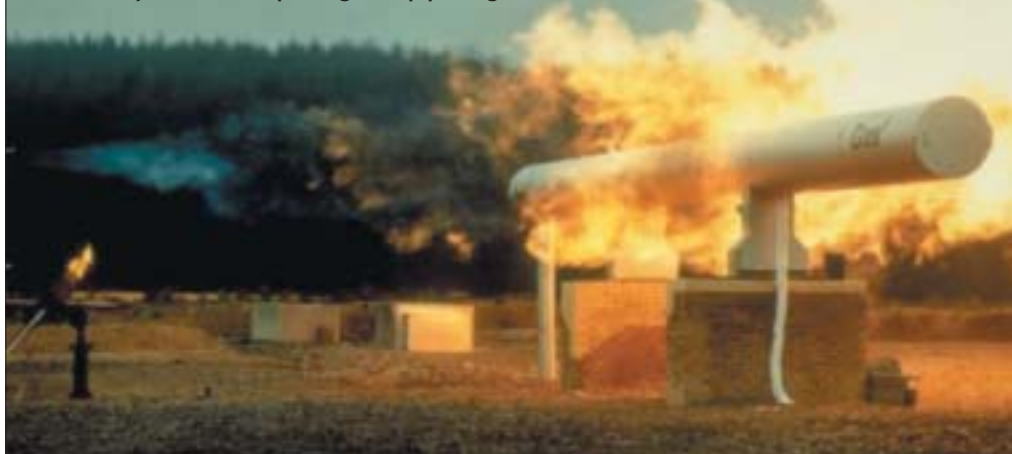
Fig 6. Unconfined jet fire test impacting on a pipe target
