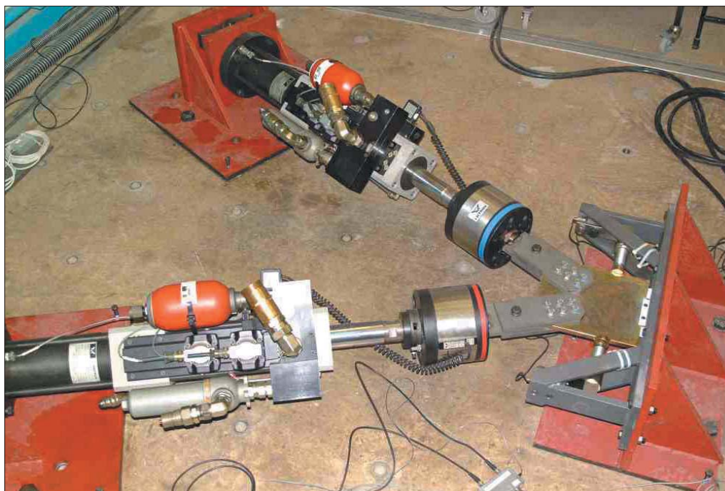
Fig 2. Test rig consisting of two small visco-elastic dampers mounted in a K-braced frame
