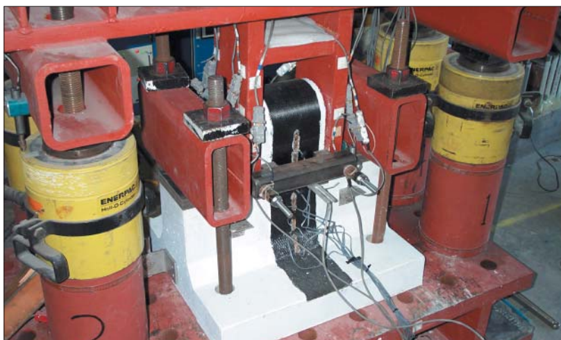
Fig 1. (Top) Arrangement for an embedded FRP anchor Fig 2. (Above) Section through typical anchor detail
