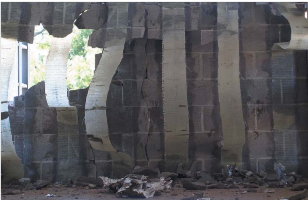
Fig 6. (Below) Un-grouted masonry wall with low level of FRP reinforcement after blast loading to 4.7psi
