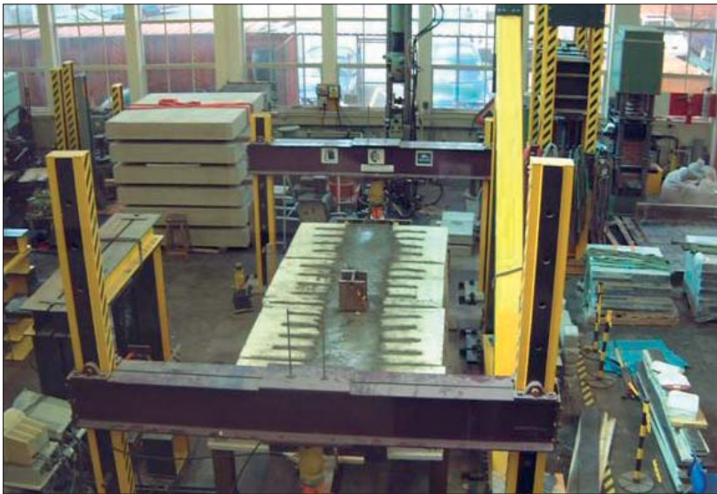
Fig 3. Beam – column connection test set-up
