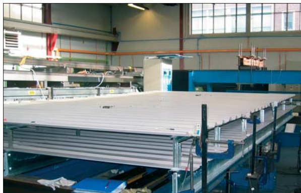
Fig 1. Built-up cladding panel undergoing structural tests
