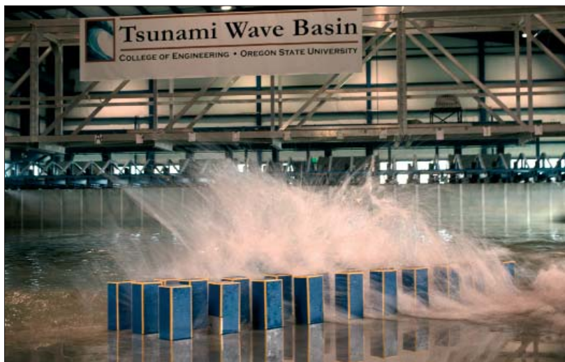
Fig 2. Demonstration of tsunami structure interaction in Tsunami Wave Basin at O.H. Hinsdale Wave Research Laboratory, Oregon State University.
