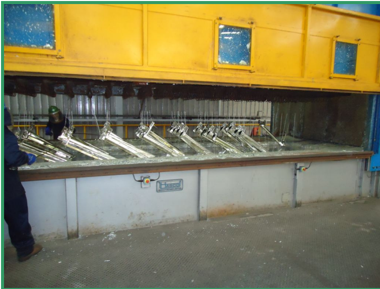
Material is being lifted out of the zinc bath and then transferred to the quench tank.
