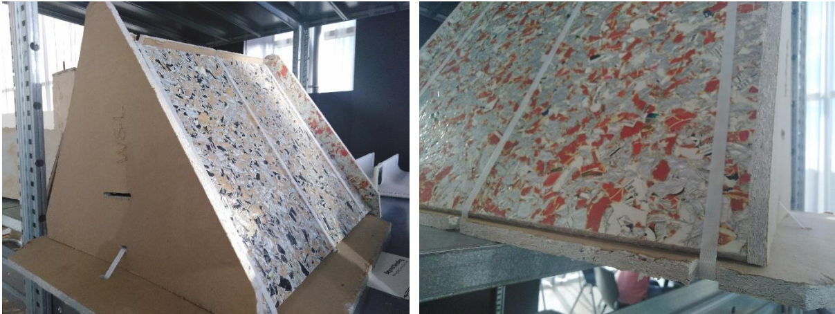
Figure 4.10 - The blocks made of recycled tetra pack boards, used for the BRG Pavilion for the Ideas City Festival 2015 in New York City.
