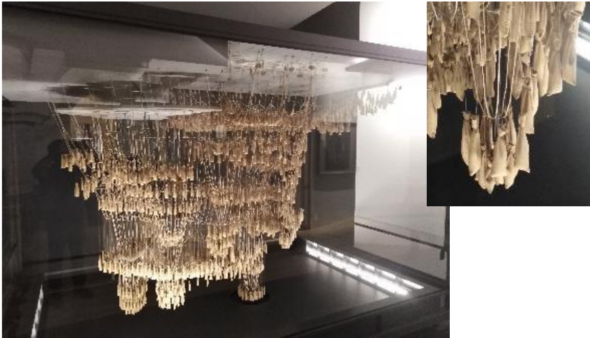
Figure 3.1 - Hanging chain model of La Sagrada Familia.
