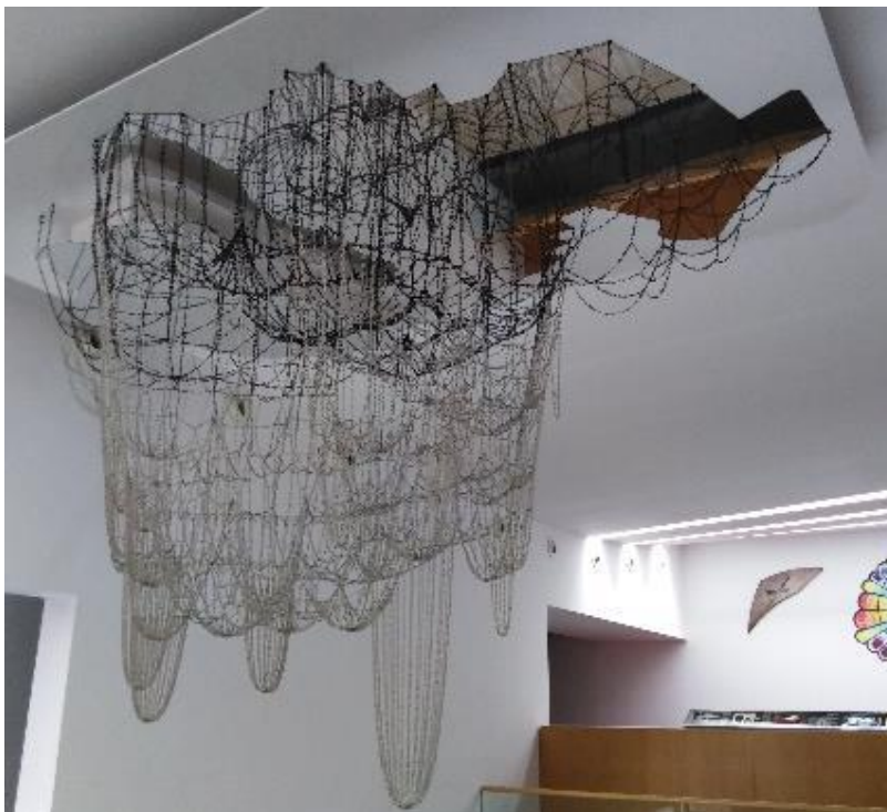
Figure 3.2 - A replica of the hanging chain model of the crypt in Colonia Güell.
