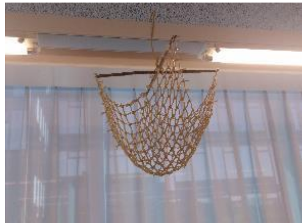
Figure 3.6 - Isler's hanging net model, with unstiffened free edges.
