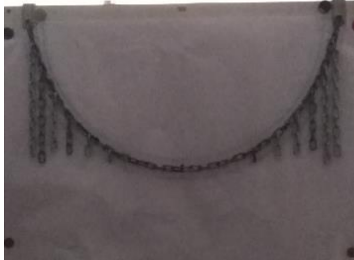
Figure 3.9 - hanging chain models used as a tool to understand optimization of vaults, as used at Auroville Earth Institute.
