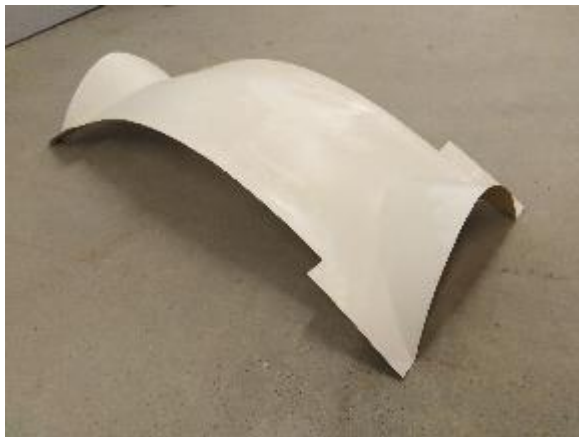
Figure 3.5 - Isler's model used for the scale model testing of the roof shell in Dübendorf Air Museum.
