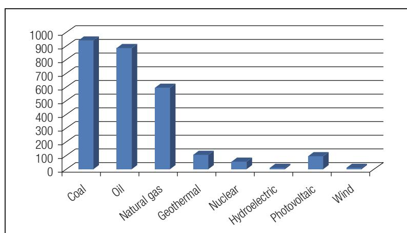
**Figure 3** Indicative levels of carbon dioxide emissions per kWh associated with different energy sources
