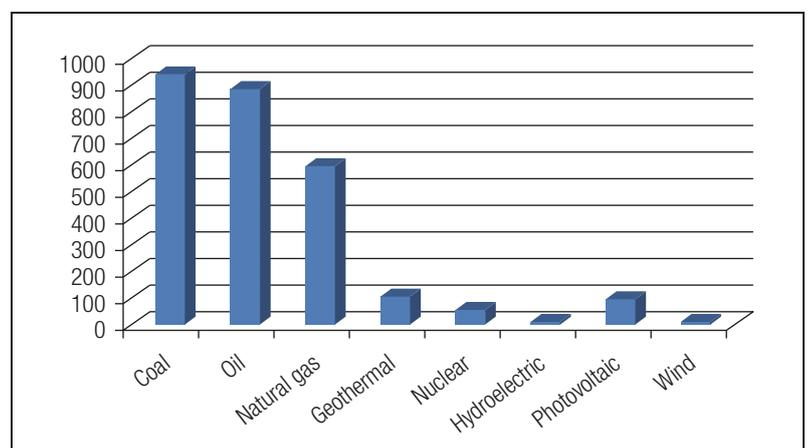
**Figure 3** Indicative levels of carbon dioxide emissions per kWh associated with different energy sources
