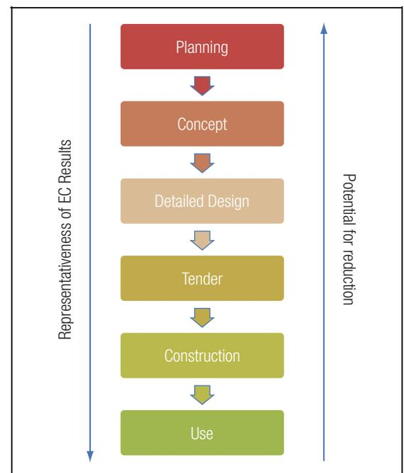
**Figure 2** In order to achieve the best results it is important that embodied carbon estimates are undertaken early in the design process, although a significant contribution can be made at every stage
