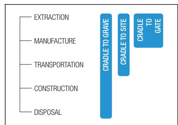
Figure 4 Schematic representation of different system boundaries
