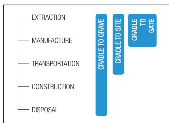
**Figure 4** Schematic representation of different system boundaries
