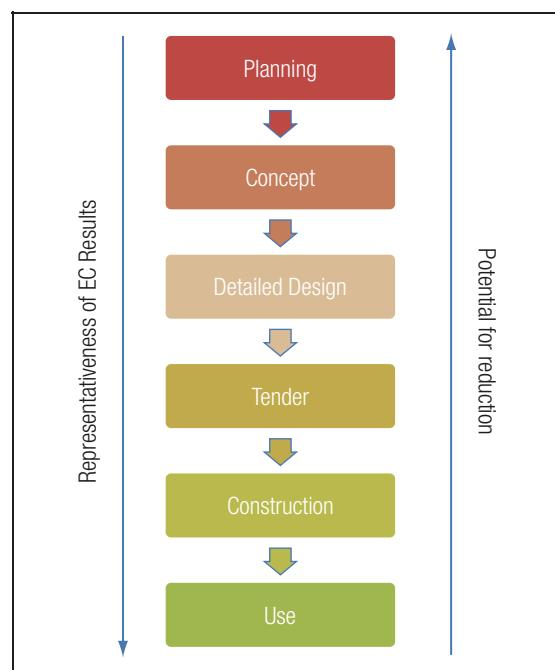
**Figure 2** In order to achieve the best results it is important that embodied carbon estimates are undertaken early in the design process, although a significant contribution can be made at every stage
