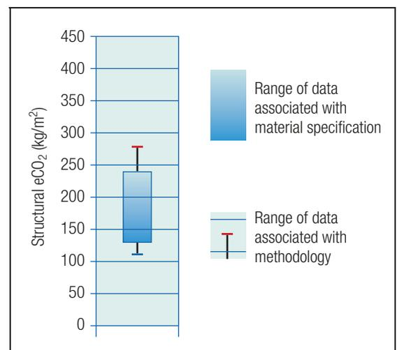
**Figure 5** Variations in the embodied carbon of the structure of a whole reinforced concrete framed building, principally as a result of differences in concrete specification (Courtesy of Arup). (The methodology for accounting for recyclability of steel and the variations in manufacturing methods used is discussed in Section 7)
