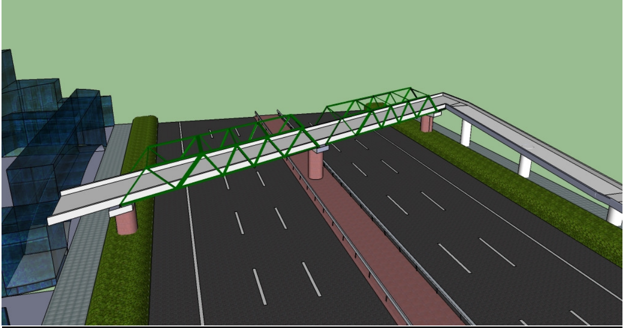
Figure 2A: Three dimensional view of the bridge concrete deck on through warren truss & ramp
