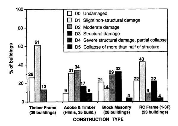
Figure 6.6 Non-cumulative damage distributions in the vicinity of the strong motion instrument
