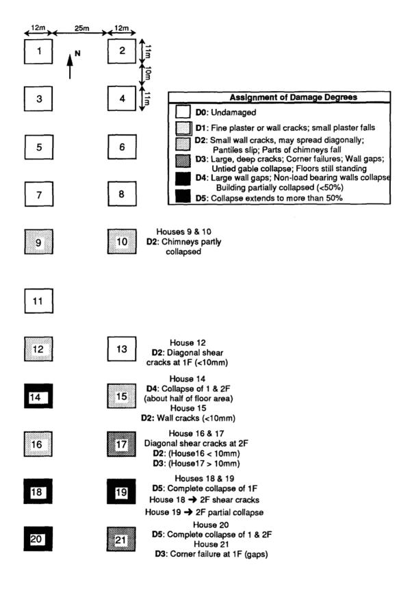
Figure 5.8 Layout of buildings on the Cooperative Housing Estate, Uzumlu, showing damage levels
