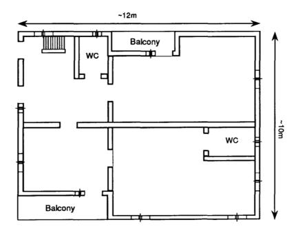
Figure 5.7 Approximate second floor plan of typical house on the Cooperative Housing Estate, Uzumlu
