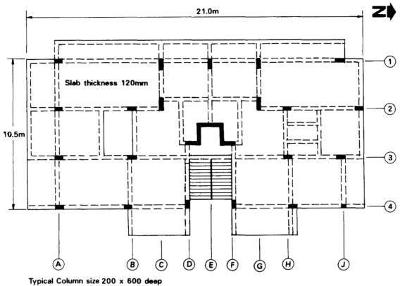
Figure 5.9 First floor plan of six storey apartment block, Bahcelievler district. Location 19.
