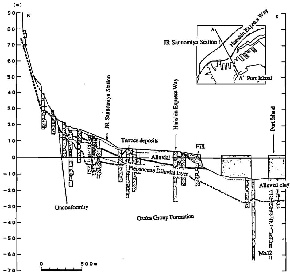
Figure 3.6 Subsurface section of Kobe (after Ishihara, et al. (1995))
