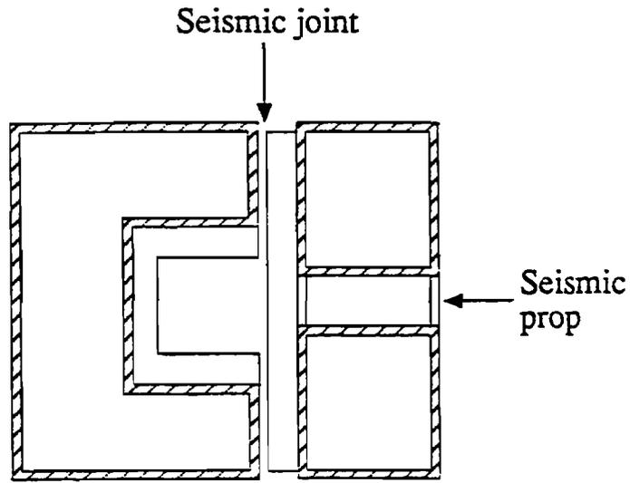
Figure 4.4 Masonry clad shear wall building
