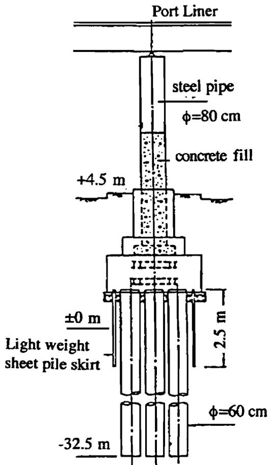
Figure 8.13 Pile foundation of the elevated Portliner Railway on Port Island (Watanabe, 1981)
