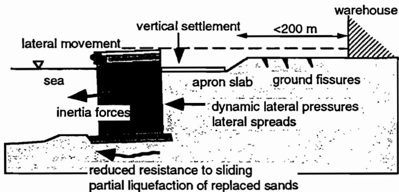
Figure 8.6 Typical damage of caisson walls
