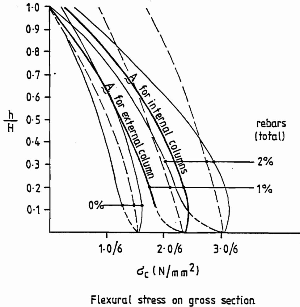
Figure 4.11 Action effect & resistance distribution with columns of constant cross-section
