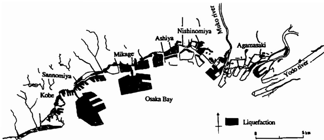
Figure 8.1 Area of liquefaction in the Osaka-Kobe region
