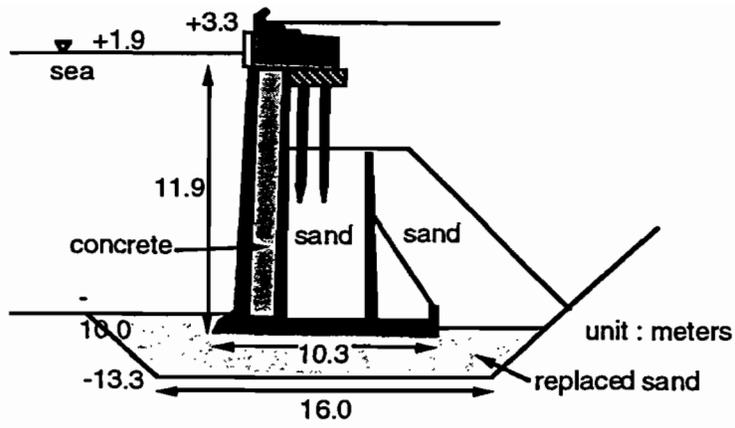
Figure 8.10 Cross-section of Shinko Pier No. 6
