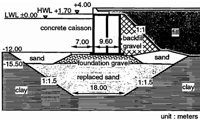
Figure 8.5 Concrete caisson wall at northeast section of Rokko Island
