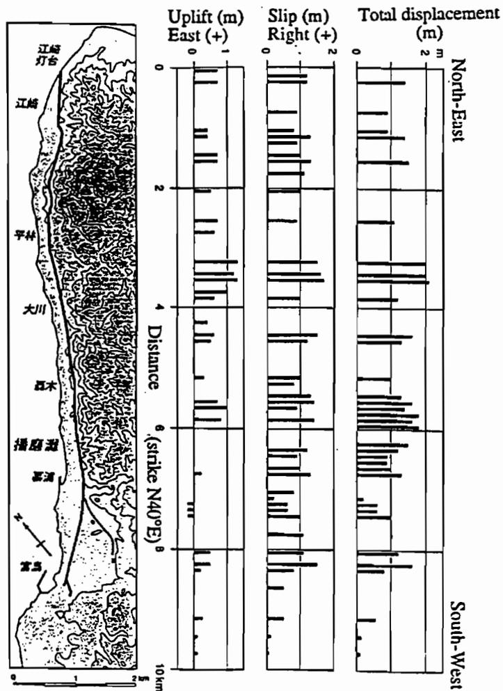
Figure 3.19 Surface displacements along the Nojima fault measured by Kurita et al. (1995)
