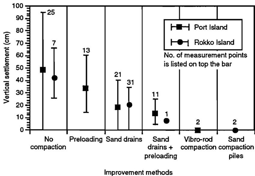
Figure 8.20 Measured vertical settlements at improved ground sites (after Mitchell, et al., 1995; Ishihara et al., 1995)
