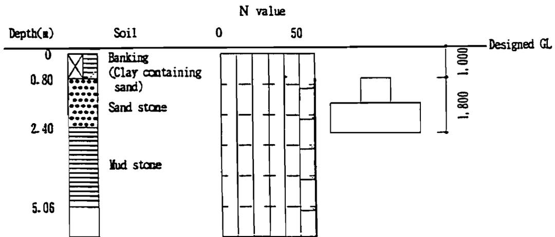
Figure 4.7 Soil profile of the MTRC building site
