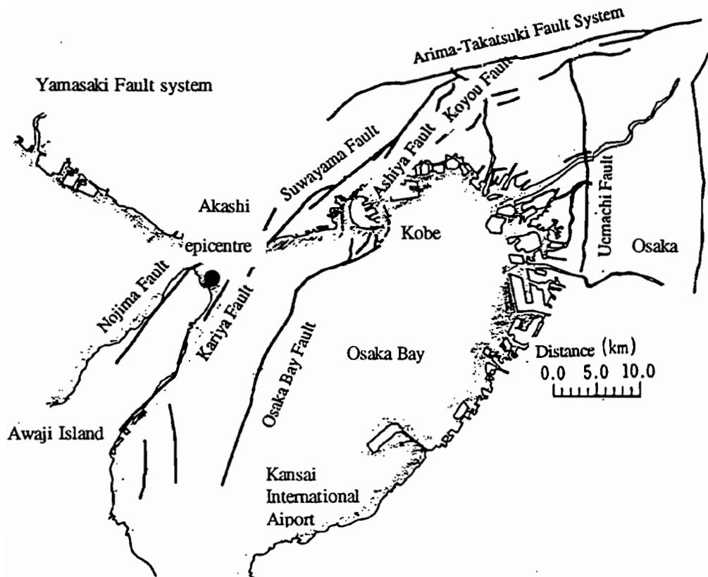
Figure 3.2 Active faults in the Kobe region (after Iwasaki (1995))
