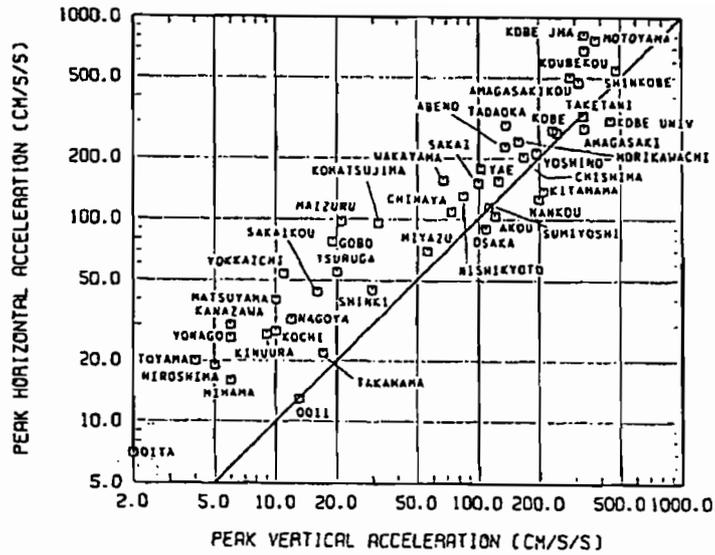
Figure 3.13 Vertical acceleration versus horizontal acceleration (after Shimizu Construction, 1995)
