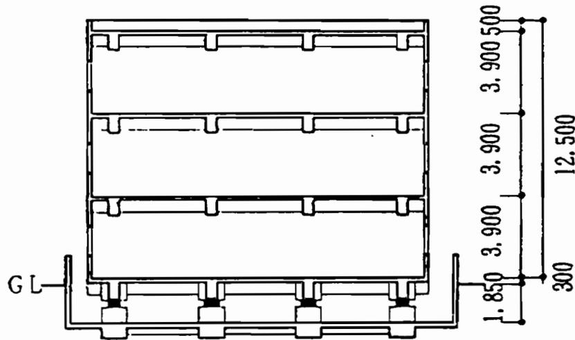
Figure 4.6b Cross-section through the MTRC base-isolated building
