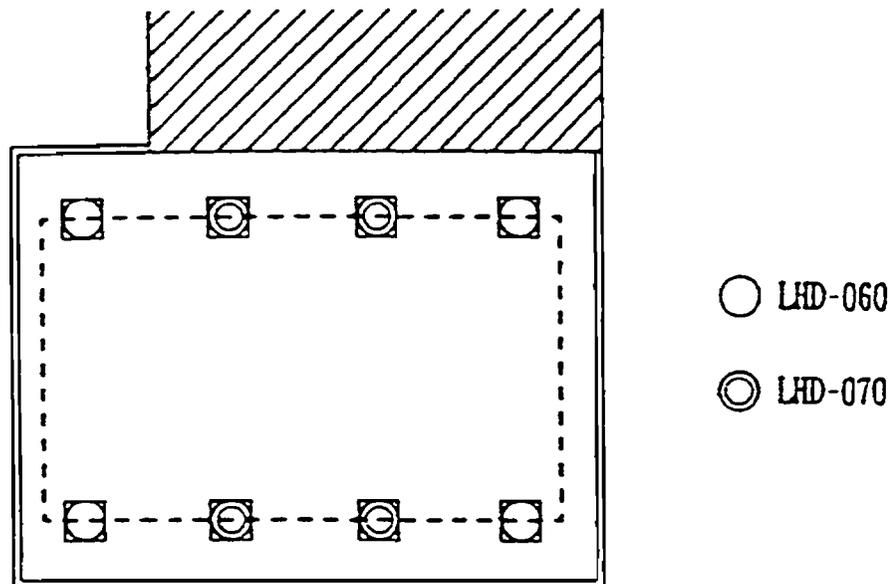
Figure 4.8 Arrangement of the isolators in the MTRC building
