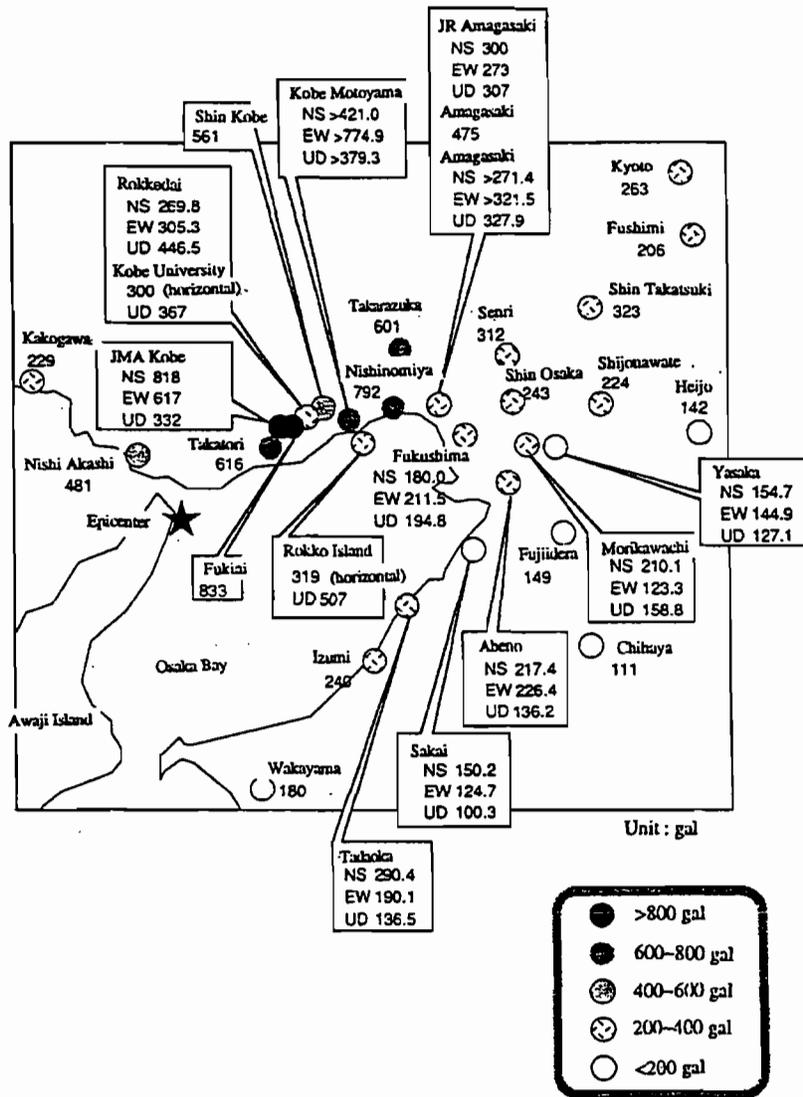
Figure 3.9 Recorded maximum accelerations (after Taisei Construction, 1995)
