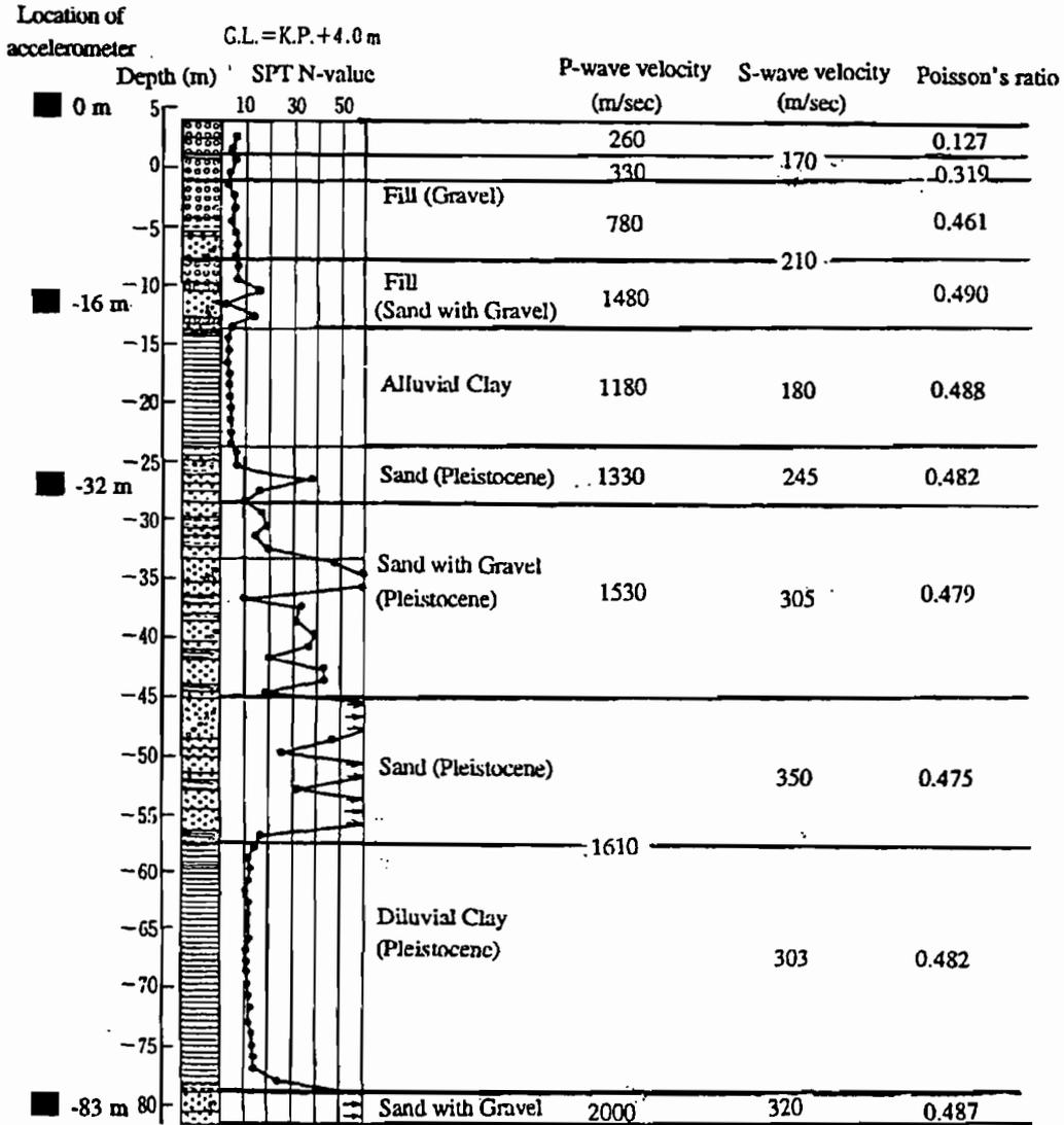
Figure 3.14 The locations of strong motion instruments at the northwest corner of Port Island
