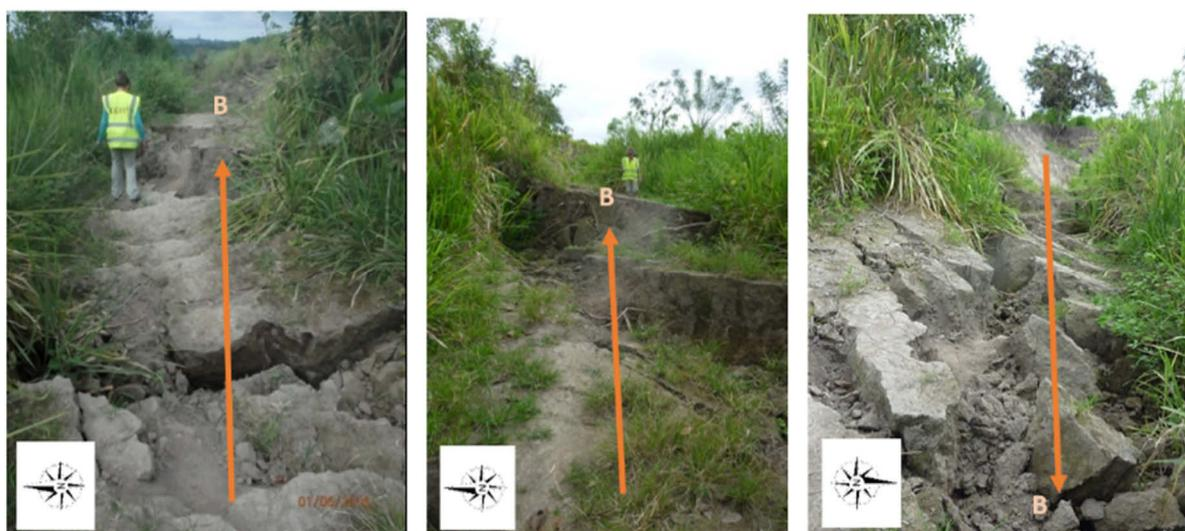
Figure 4-20 San Isidro site A, rotation and translation of surficial blocks of soil close to the head of the slope. Photo taken of ground along the path defined as (B) on panoramic picture above.
