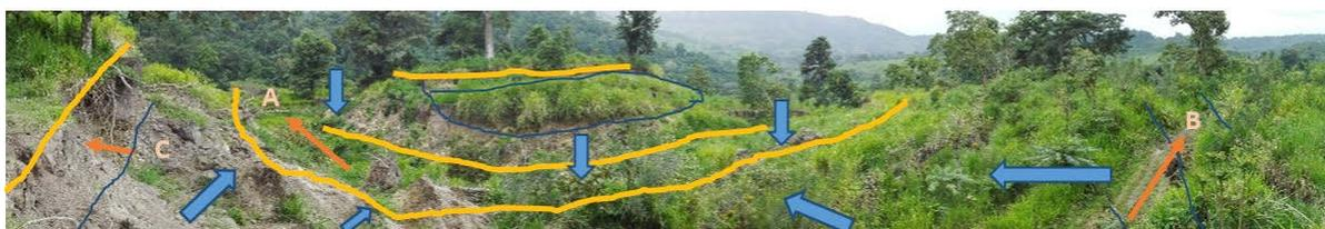
Figure 4-18 Panoramic view of the ground failure at Site A (yellow lines indicate primary scars, and blue ones the secondary ones; the blue arrows show the movement of the soil).
