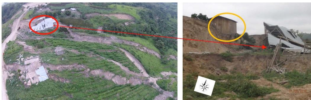
Figure 4-22 San Isidro site B, taken from a drone. A river runs through the trees at the bottom of the slope, to the right of the figure (the yellow circle shows the intact house next to the slope that failed).
