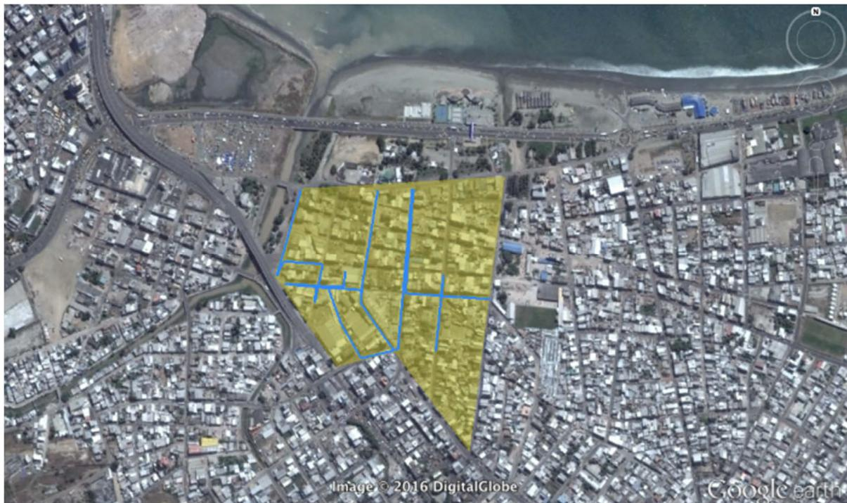
Figure 6-21 Survey routes (blue lines) in the restricted zone (yellow shaded area) in Tarqui, Manta. Centre of image: (-0.9535, -80.7149).
