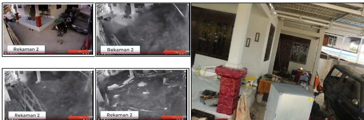
Figure 6.11 - Video frames at 18:03:01, 18:06:29, 18:06:30, 18:06:36 and during the EEFIT mission. Notice the mopeds have fallen over, following by the bore-like tsunami about 3 minutes later. This short arrival time supports the argument, discussed in Section 6.2.1, for a secondary tsunami source within Palu Bay.
