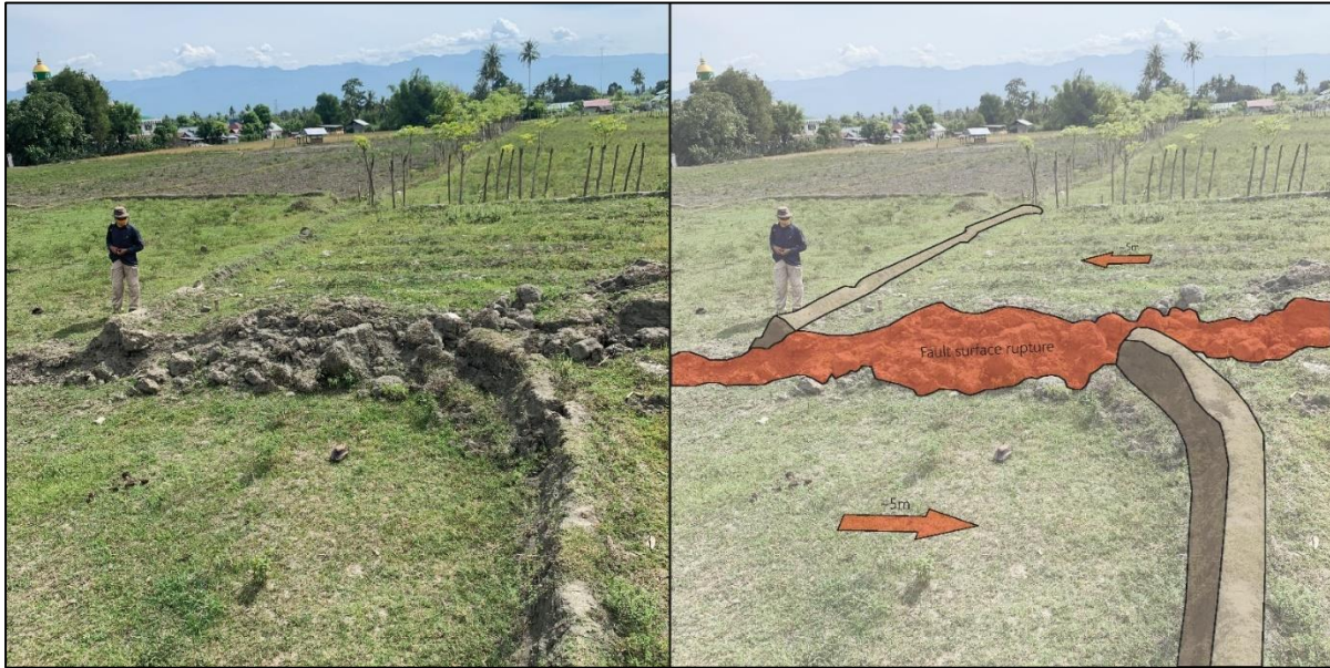
Figure 3.6 – Displacement of approximately 5m along fault surface rupture shown due to offset rice paddy terraces.
