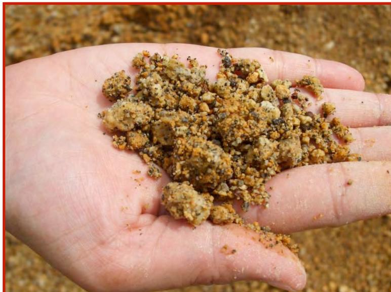
Figure 66. Weathered pumice collected from the landslide debris.
