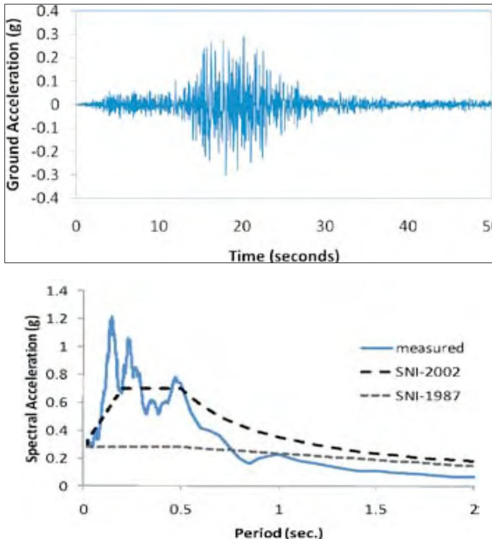
Figure 10. Ground acceleration and response spectra (N-S component) and design earthquake spectra (EERI, 2009).
