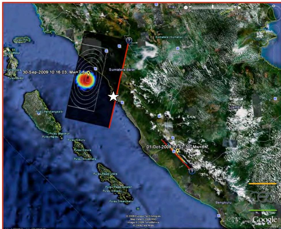
Figure 9. Fault plane proposed by the CEA for the 30<sup>th</sup> September Mw 7.6 Padang earthquake. The star shows the location of Padang. Note the calculated fault plane of the 1<sup>st</sup> October Mw 6.8 earthquake to the Southeast of the largest event.
