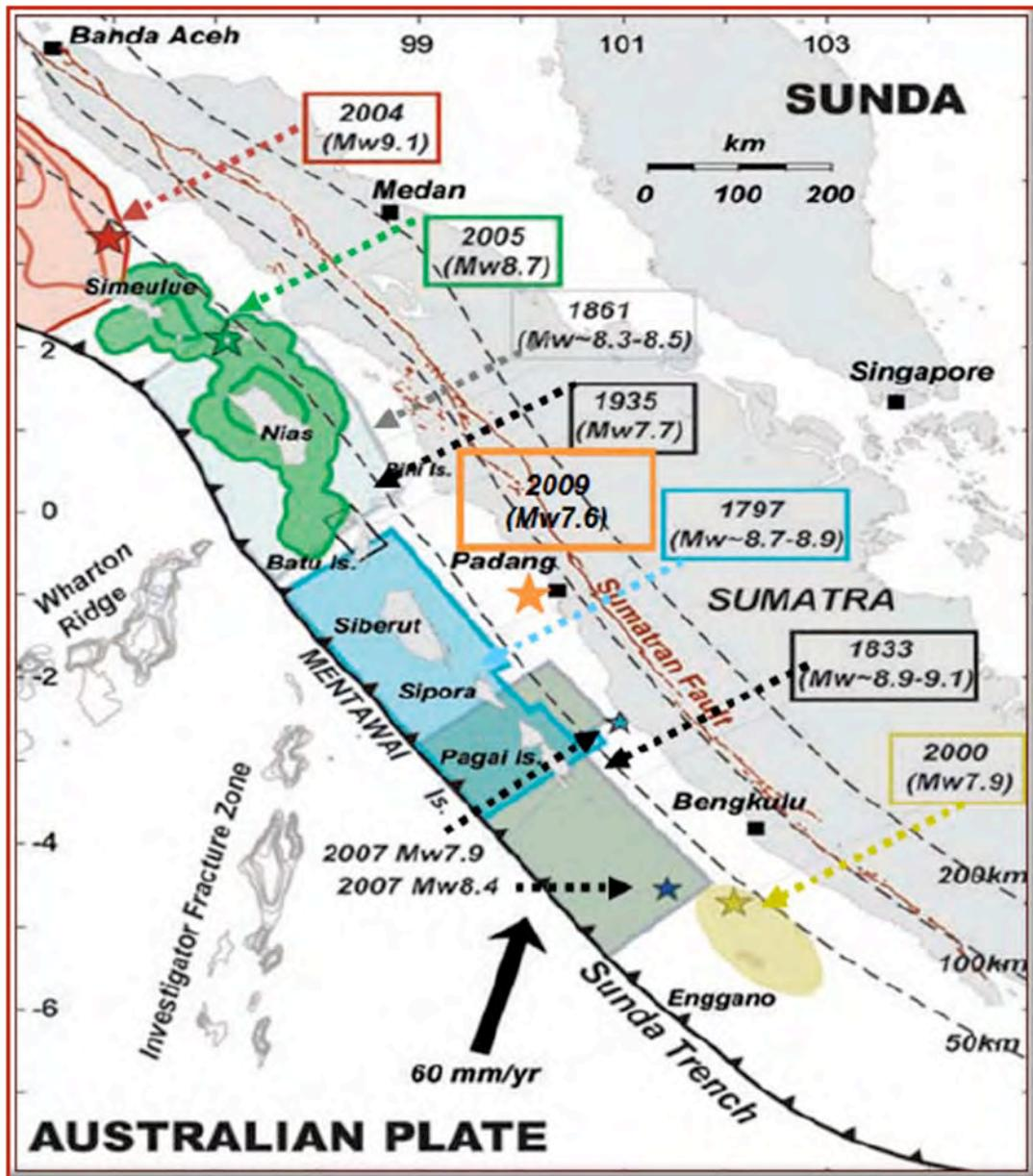
Figure 7. Large events in the Sunda trench along Sumatra and their associated rupture areas (Chlieh et al., 2008). Note a recent seismic gap between the 1833 and 1861 events, on the region where the 1797 event occurred. The star shows the epicentral location of the event.
