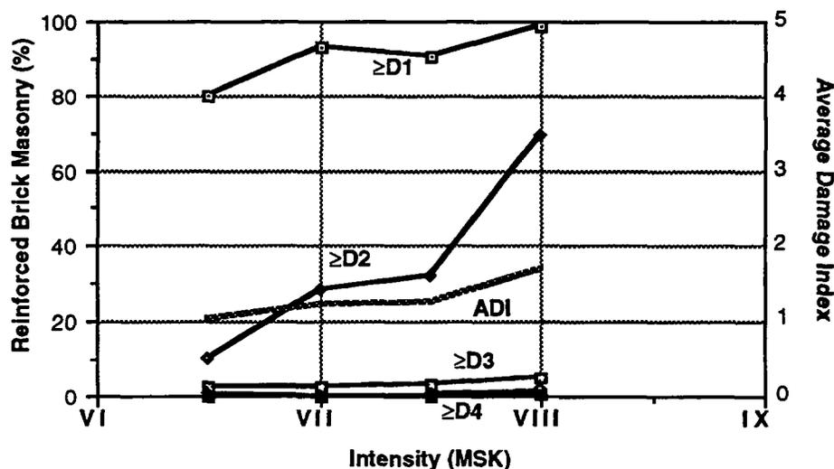
Figure 10: The vulnerability of low-rise reinforced brick masonry buildings, built before 1940 (Bucharest, 1977 earthquake).
