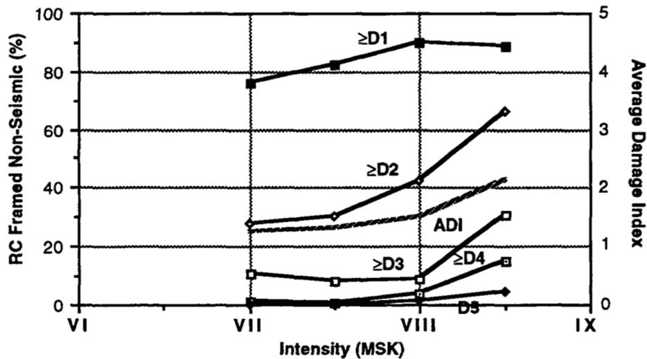
Figure 13: The vulnerability of the old RC framed apartment buildings (Bucharest, 1977 earthquake).
