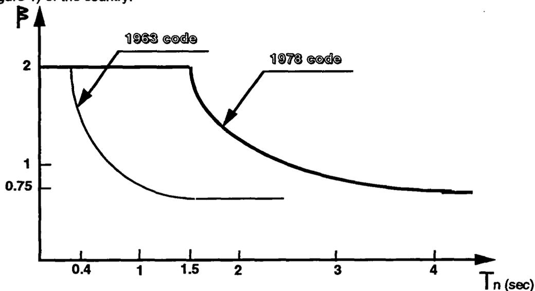
Figure 5: The effect of changes with the introduction of the 1978 code, upon the amplification factor ( $\beta$ ).
