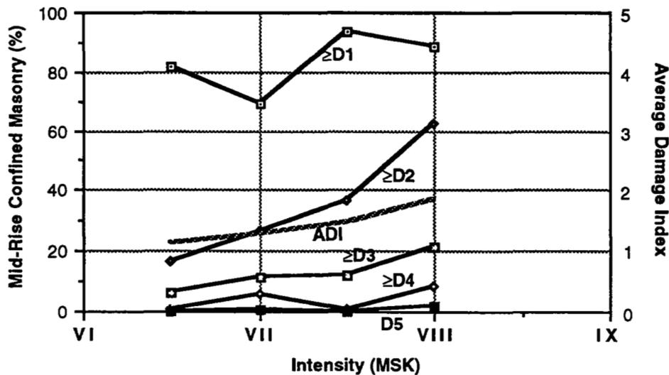
Figure 11: The vulnerability of mid-rise confined brick masonry buildings (Bucharest, 1977).
