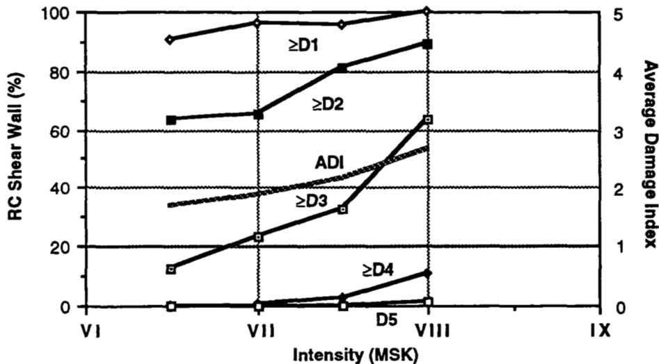
Figure 14: The vulnerability of multi-storey RC shear wall apartment buildings (Bucharest, 1977 earthquake).
