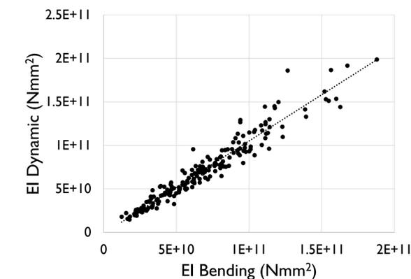
For EI Bending (flexural stiffness) against EI Dynamic, the correlation coefficient was  $R^2=0.932$  and for EI Bending vs Max Bending Moment (flexural capacity), the correlation was found to be  $R^2=0.851$ .
