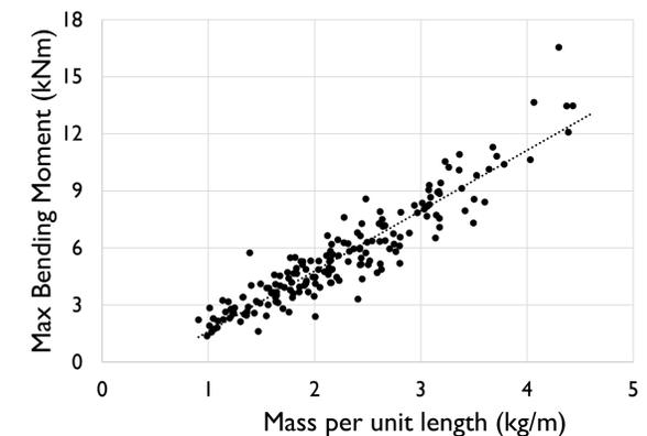
In particular, mass per unit length and average external diameter were found to be good indicators of strength with high  $R^2$  values as shown in the tables below.
