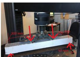
Four-point flexural test
