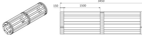
Optimum designed truss for lab test
