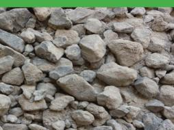
Figure 4. RCA after LA abrasion test
