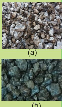
Figure 2. Aggregates coated with waste plastic
