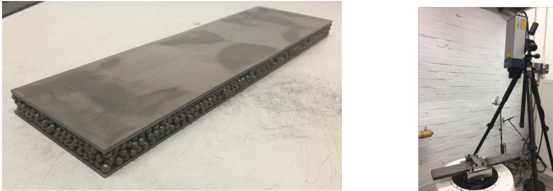
Figure 1 (a) – A SFS4 specimen. (b) – Experimental set up for vibration testing.
