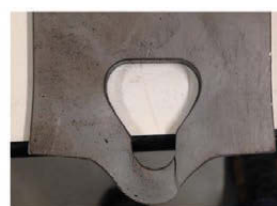
(b) E1-1.5 (Shearing and bearing)
