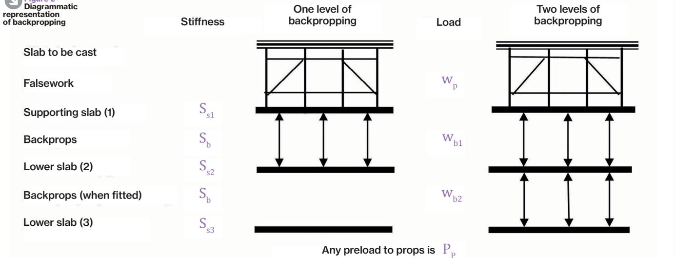
act as a distributed load, or as individual point loads from each of the falsework legs? Further, the grid of backprops below the supporting slab, transferring load to lower floors, will rarely be at the same centres as the falsework legs (only about a third of the load is transferred); hence, the concrete supporting slab will also have an influence on load transfer.
