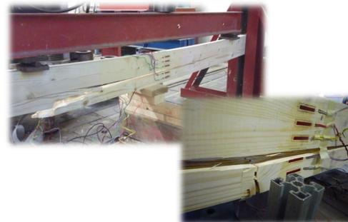
Example tensile failures at knots in control beams
