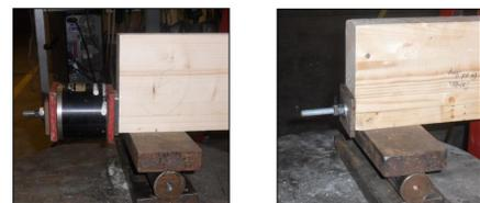
Load cell & Steel pressure plates secured in place
