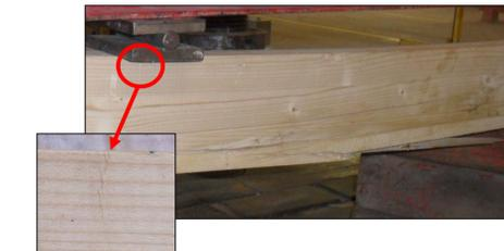
Example of initial compression failure of 10kN prestressed beams
