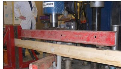
Spreader beam used to transfer point load to 1/4 points of test beam
