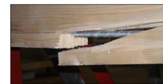
With an increase in stress induced in the tension region of the beams the strength of finger joints became critical
