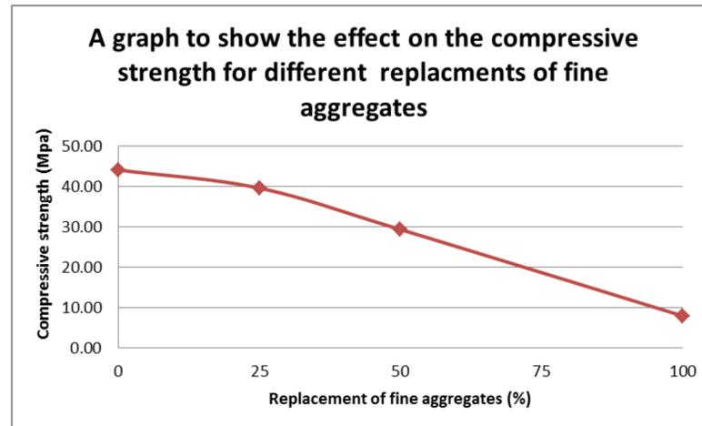
It can be seen from the graph on the left that the replacement of fine aggregates with plastic had a dramatic effect on the compressive strength of the concrete. As the percentage of plastic replacement increased, the compressive strength decreased significantly. This was due to the plastic particles not being able to create a strong bond with the cement paste.
