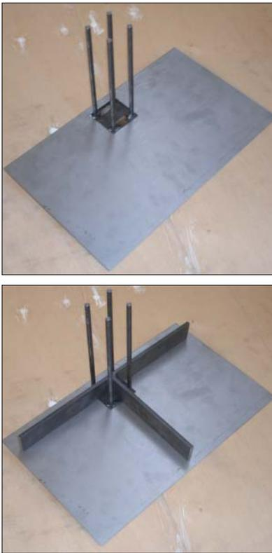
**Fig 3. Construction stages of edge column-slab detail for test**
