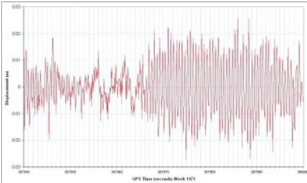
Fig 2 shows a number of spikes in the vertical displacement that coincided with the periods of people jumping on the bridge. These spikes were then investigated further, (see Figs 3 and 4) and the vertical residual displacement plotted for time periods of one minute.
