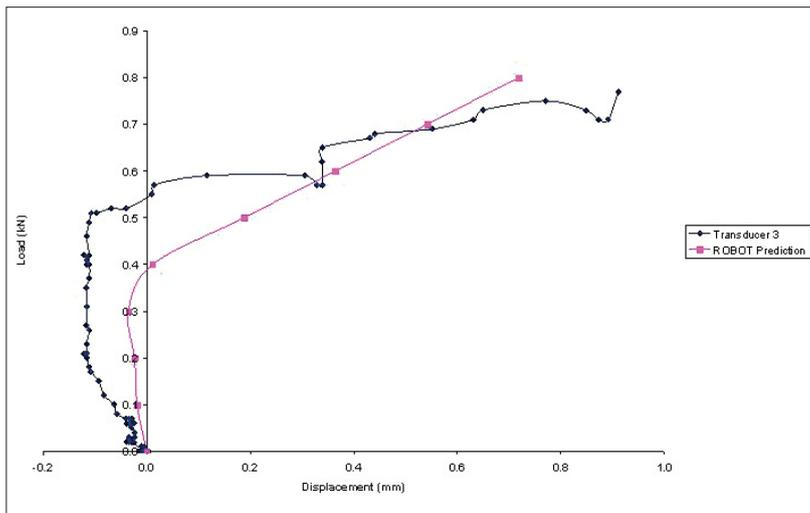
Fig 7. Prediction superimposed upon test frame result
