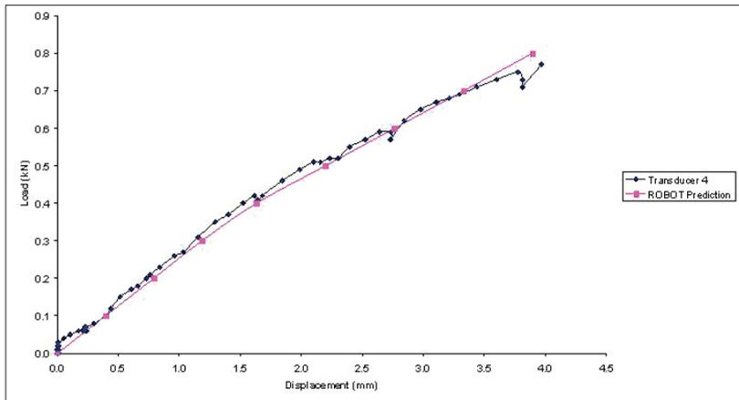
Fig 6. Prediction superimposed upon test frame result
