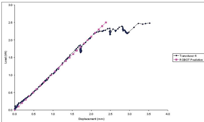
Fig 8. Prediction superimposed upon test frame result
