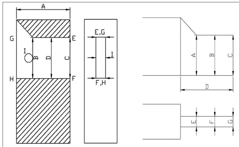
Table 1: Test Connection Dimensions for Tenons corresponding to Fig 1
