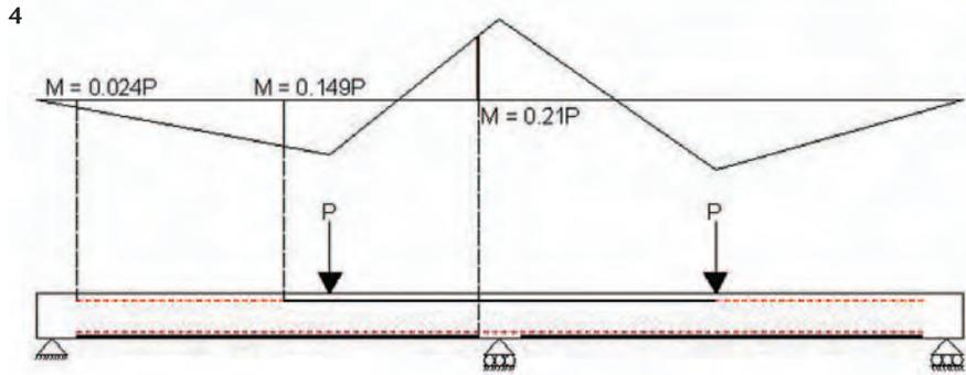
Fig 3. Location of failure planes in a typical section / Fig 4. Potential extension of anchorage zones to avoid separation failure
