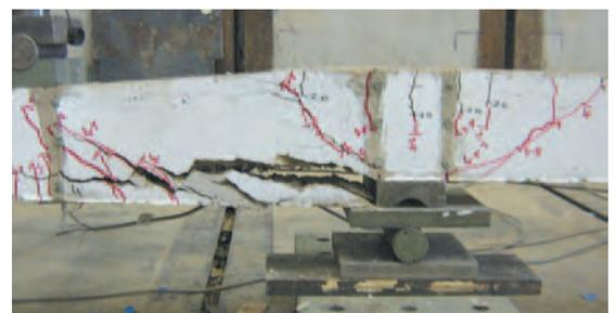
Fig 1. Test set up (Beam 2 shown) / Fig 2. Concrete cover separation failure in Beam 3
