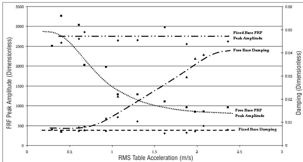
Therefore, in this experiment, a factor 5 increase in system damping should correspond to a factor 10 decrease in the peak deformation response factor.
