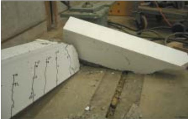
Fig 5. Catastrophic failure of Beam A
