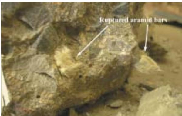
Fig 6. Dowel rupture of beam B (detail)
