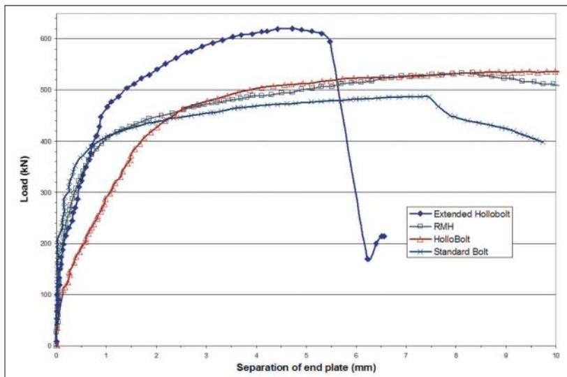
**Fig 5.** Load-displacement relationships, normalised for ultimate load of standard bolt
