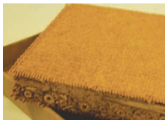
Fig 9. The Vikas Community, an example of Stabilised Earth Masonry, Auroville / Fig 10. Combination of RC frame and earth blocks (Agdz, Morocco) Fig 11. Top left: Light earth (expanded kaolin), provides the advantage of improving thermal insulation in comparison to denser earth blocks, and is less prone to result in cracking. bottom left: Unfired, non-stabilised dense loam bricks used with clay mortar. Right: Light earth and unfired brick masonry infills to timber frame. For light earth, the procedure requires the use of shuttering on both sides / Fig 12. Some CLAYTEC products: loam for plaster (top), fibre loam board (bottom left) and earth blocks of different densities (bottom right)
