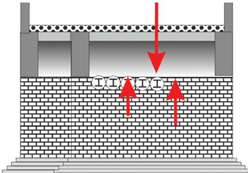
Figure 22 Cross section of pier showing needle positions and construction joint
