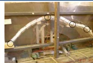
Hinge points on failed skew FlexiArch - mechanism formed - sustained 22.9kN
