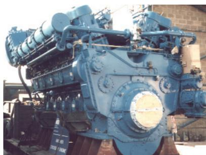
A CHP engine awaiting installation on its foundation block within a plant room
