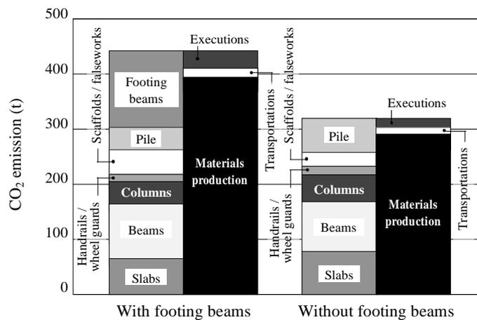
Fig. E-2: CO<sub>2</sub> emission of RC rigid frame viaduct
