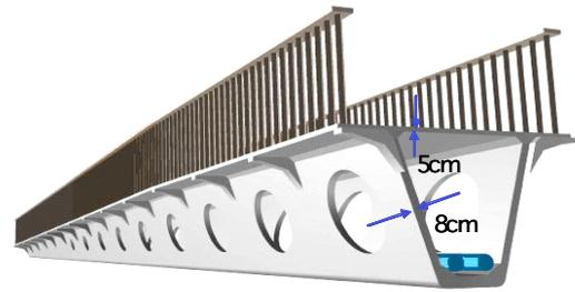
Fig. E-5: Sectional view of UFC bridge
