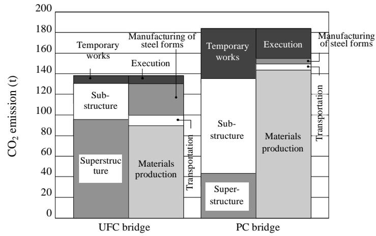
Fig. E-7: CO<sub>2</sub> emission of UFC and PC bridges
