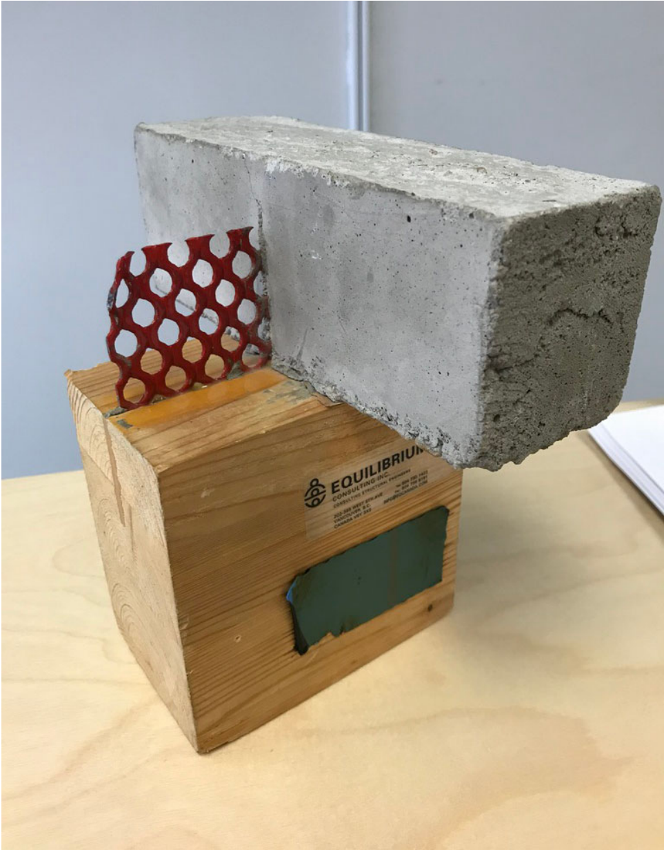
Figure 11: HSK timber-concrete composite connection
