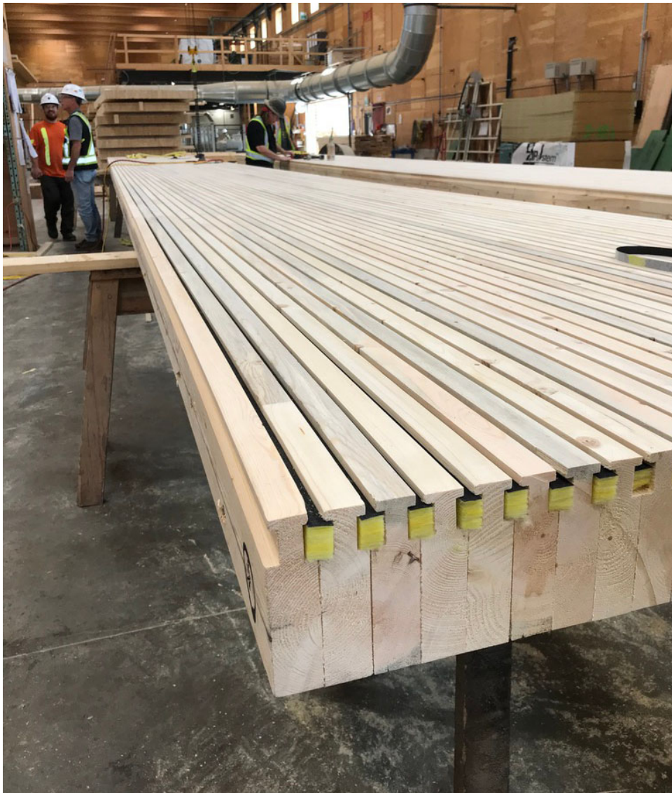
Figure 4: DLT panel during production at StructureCraft
