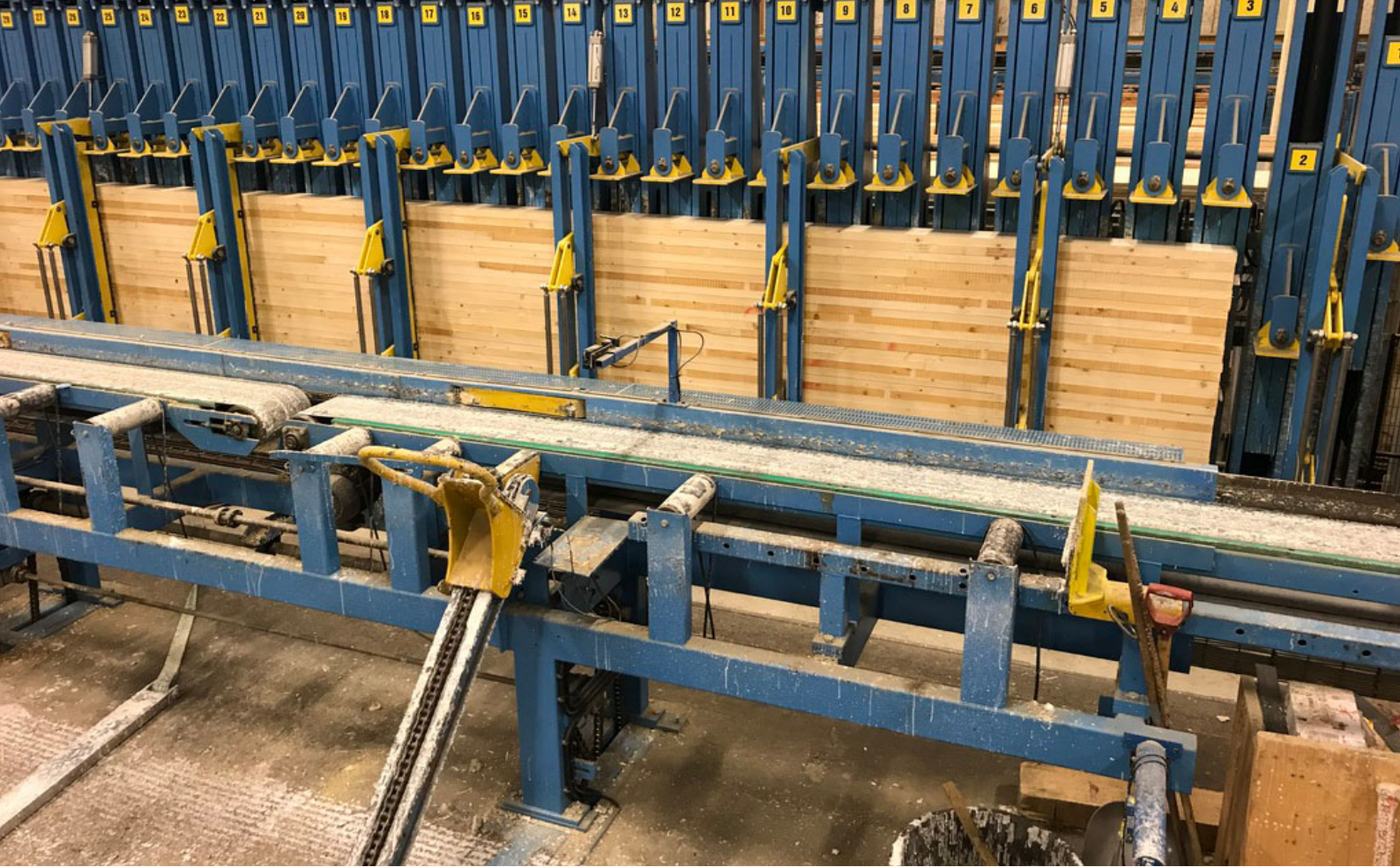
Figure 25: Glulam press at Moelven glulam factory, Norway
