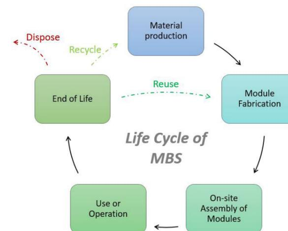
**Fig 2** Life Cycle of Modular Building System (MBS)
