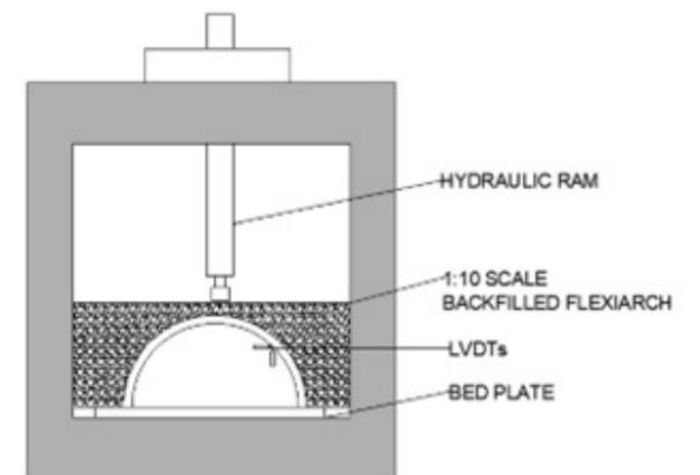
Fig 2 Scale model under the Small Dartec Machine
