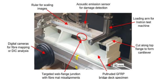
Fig. 1 GFRP deck cantilever testing set up
