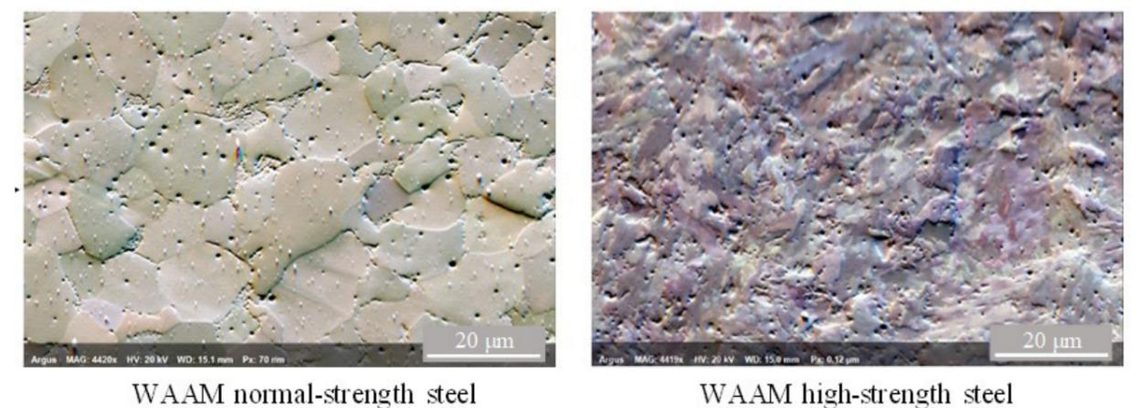
Fig 2 Typical microstructure of examined WAAM steels
