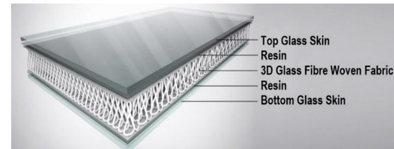
Fig 1 Schematic diagram showing the Glass-GFRP sandwich.
