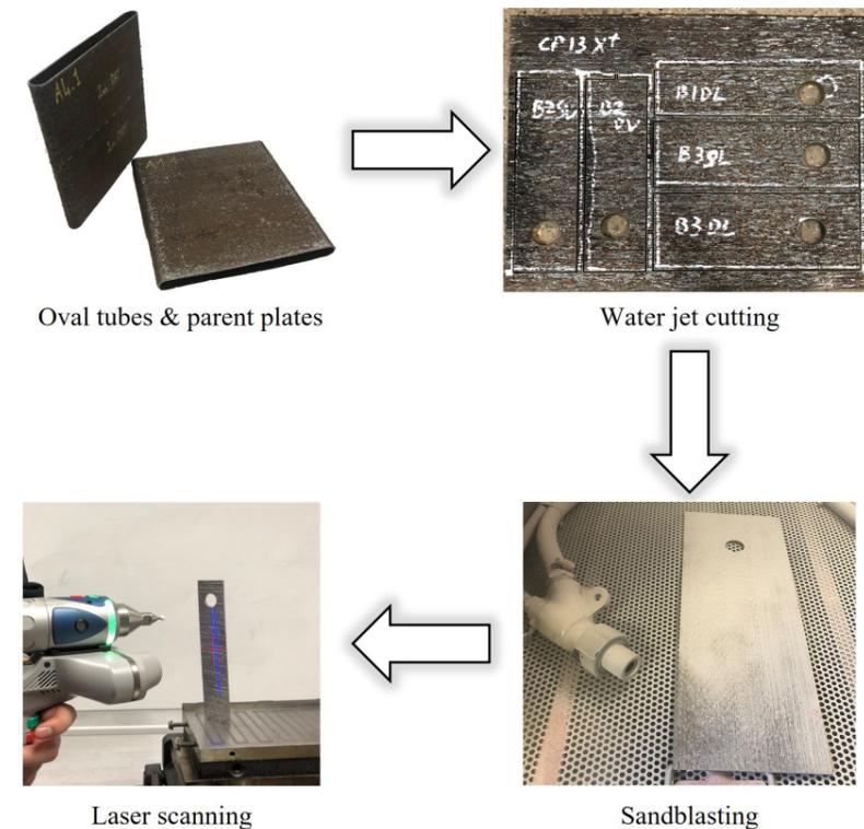
Fig1 Specimen preparation
