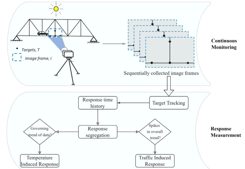
Fig 1 Vision-based thermal response measurement method
