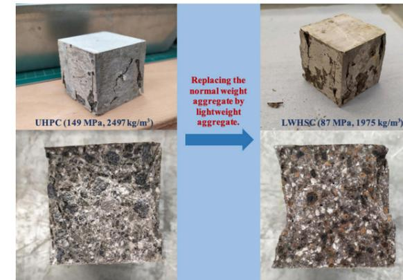
Fig 1: Development of LWHSC from developed UHPC mix
