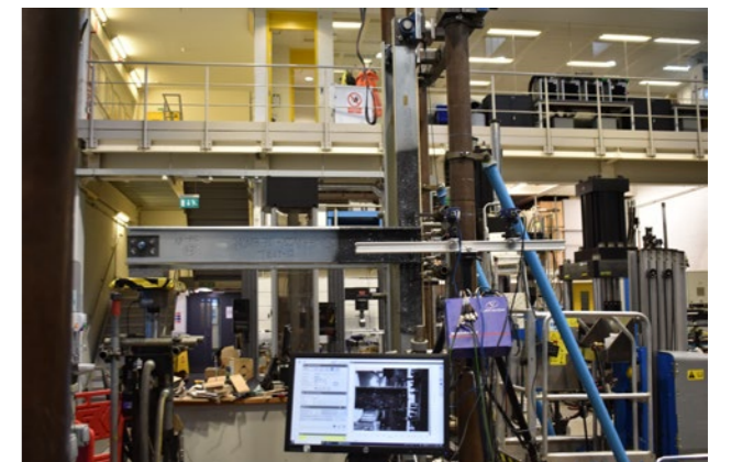
Fig 1 Experimental layout of T-frame tests (Structures Laboratory, Imperial College London)
