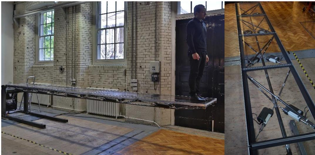
Figure 3: Loaded adaptive truss with zero deflection (left); actuators integrated (right).
