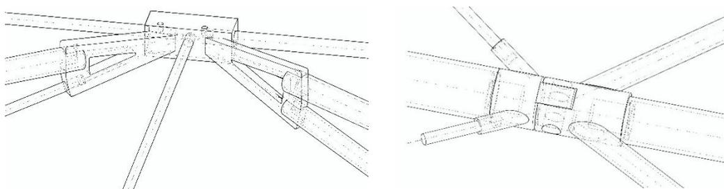
Figure 2: top cord joint (left); bottom cord joint (right);
