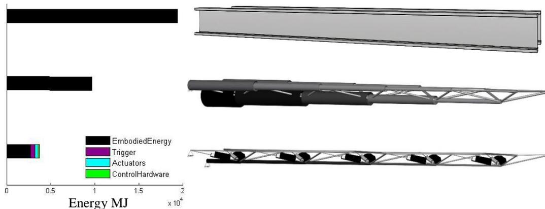
Figure 5: energy comparison (a) I-beams (b) optimised passive truss (c) adaptive truss
