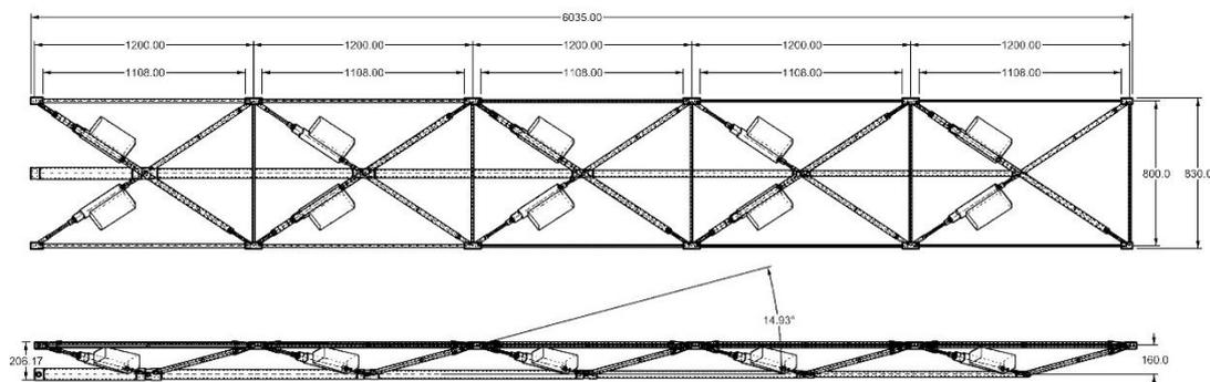
Figure 1: Adaptive truss plan and elevation with overall dimensions (mm)
