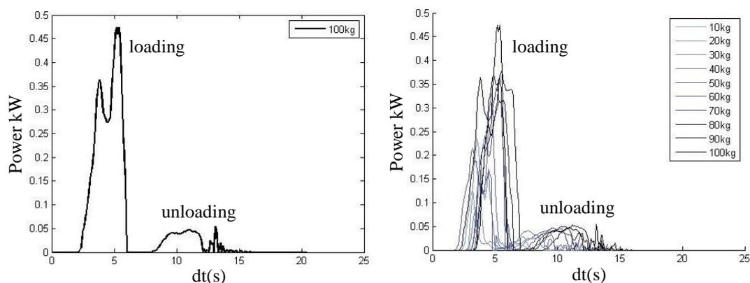
Figure 4: Power measurements (current sensor)
