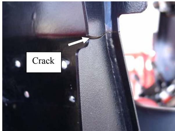
Figure 5. Fatigue crack in seat
