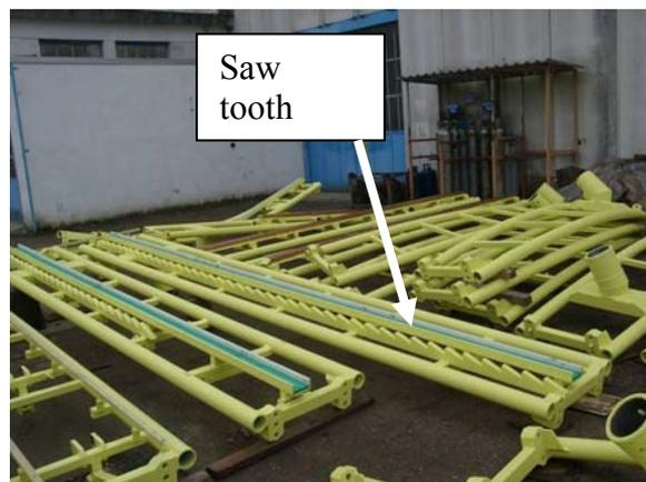
Figure 6. Anti roll-back devices.
