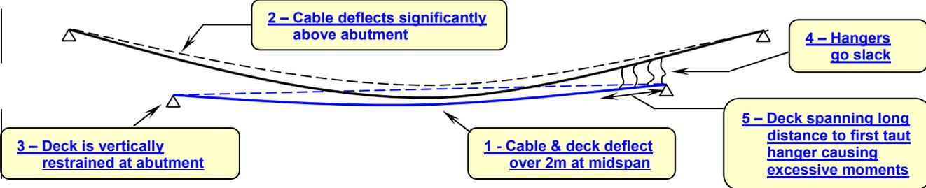
Figure 4. Structural effects of main cable ‘oversail’ (uncorrected).
