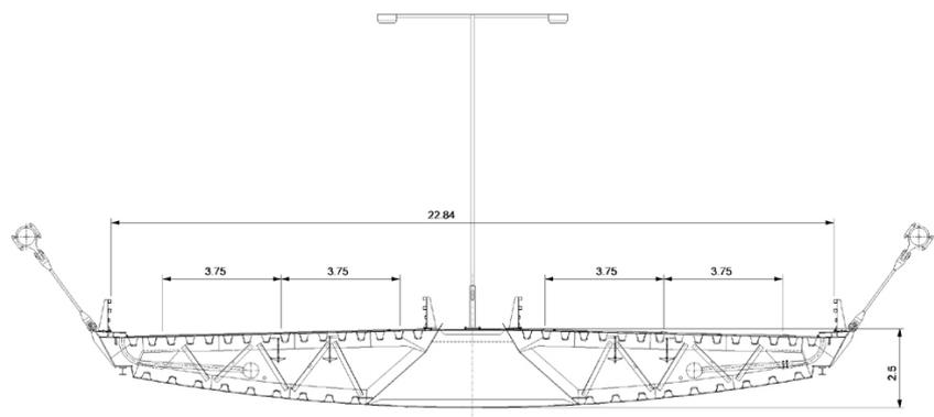
Figure 3. Deck cross-section
