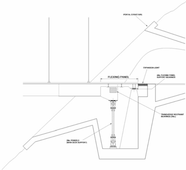
Figure 5. Articulation of deck end at abutment.
