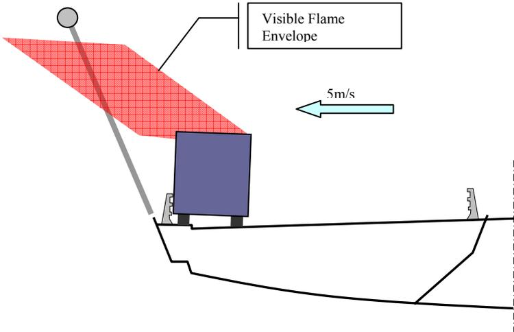
Figure 6. Visible flame envelope of design vehicle fire at 550 °C.
