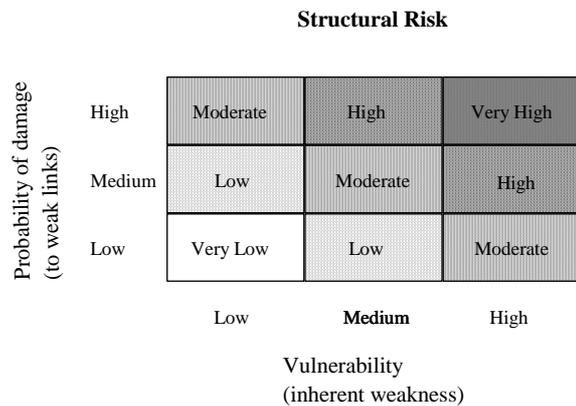
Figure 2. Structural risk as a function of vulnerability and probability of damage
