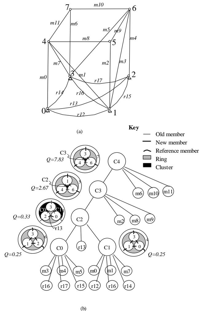
Figure 3. (a) An example structure and (b) its hierarchical model (along with graphical description of clusters)
