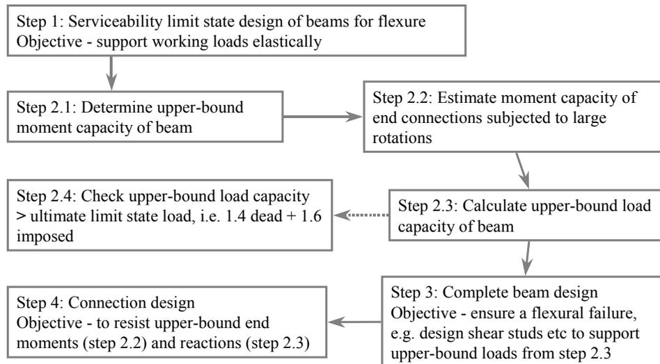
Fig. 4: The alternative design approach
