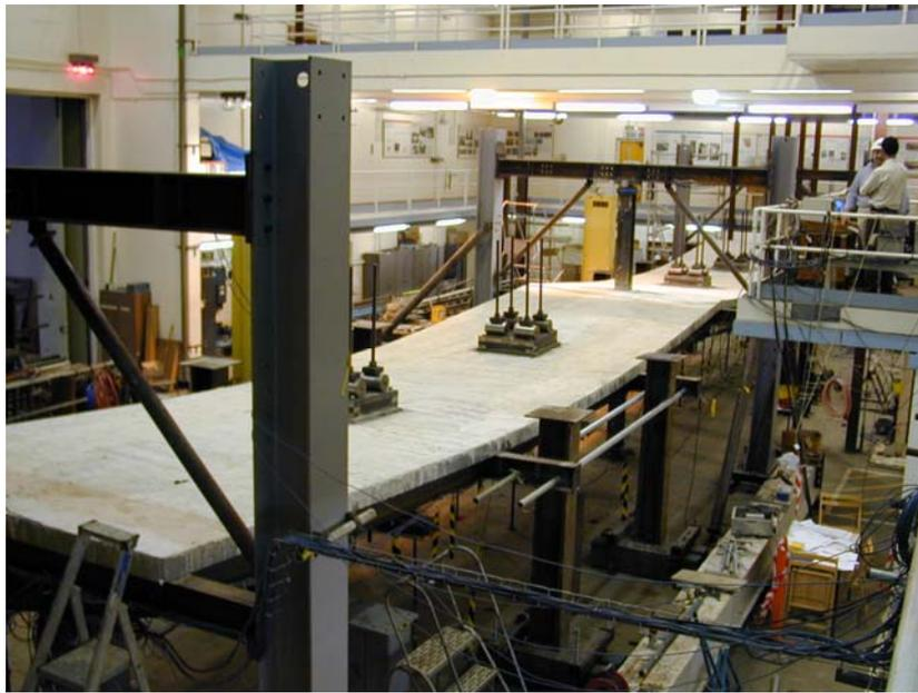
Fig. 2: Composite beam test at BRE
