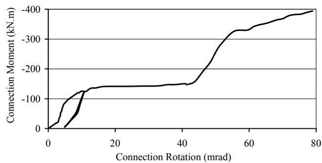
Fig. 3: Moment vs. rotation curves for partial depth flexible end-plate connection
