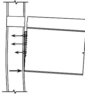
Fig. 1: Behaviour of partial depth flexible end-plate connection subjected to large rotation
